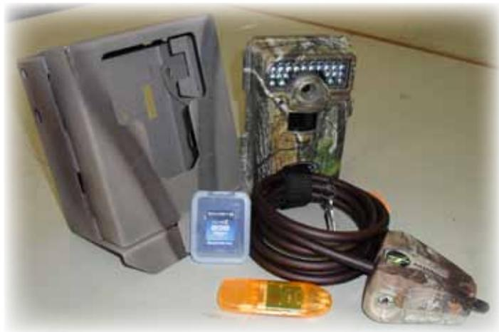
Each camera comes with a camouflage metal security box and security cable. Images are stored on an 8Gb SD card. Data from the card can be displayed and uploaded to PC via an SD card reader (both the card and reader are provided as part of the loan equipment).
