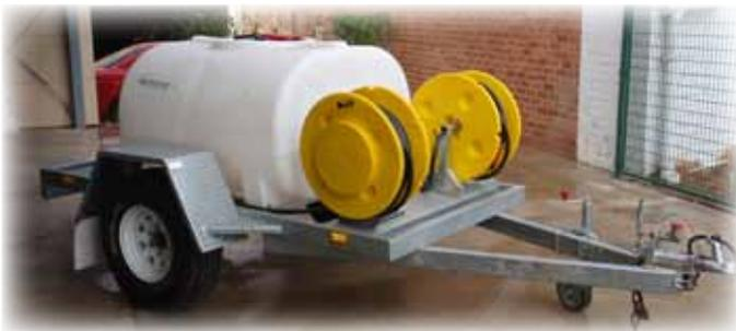
Our water trailer has a 1000L capacity and can be towed by a standard vehicle or tractor. The trailer has been constructed with rough terrain in mind. Large 4WD tyres, heavy duty
